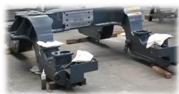
Loco Bogie Frame- Queensland Railways
