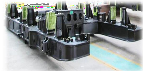
Loco Bogie Frame- Queensland Railways
