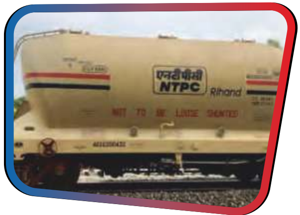
BTAP wagon for carrying, alumina and flyash
